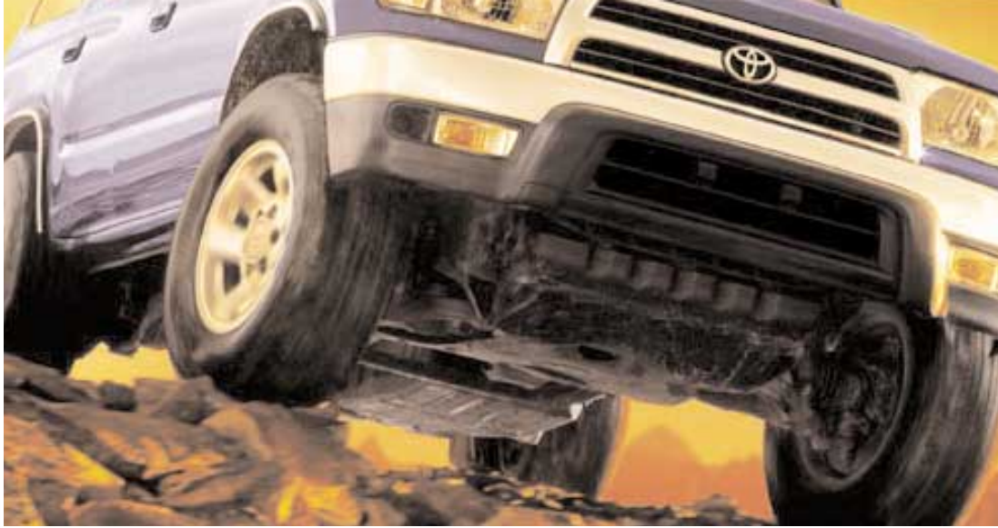
A strong coil-spring, double-wishbone front suspension provides lots of wheel travel – a major benefit to rock crawlers and highway commuters alike. Complementing this design is a solid-axle 4-link/coil spring rear suspension.
